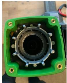
Remove the piston ring, and mount on the new driver blade.
