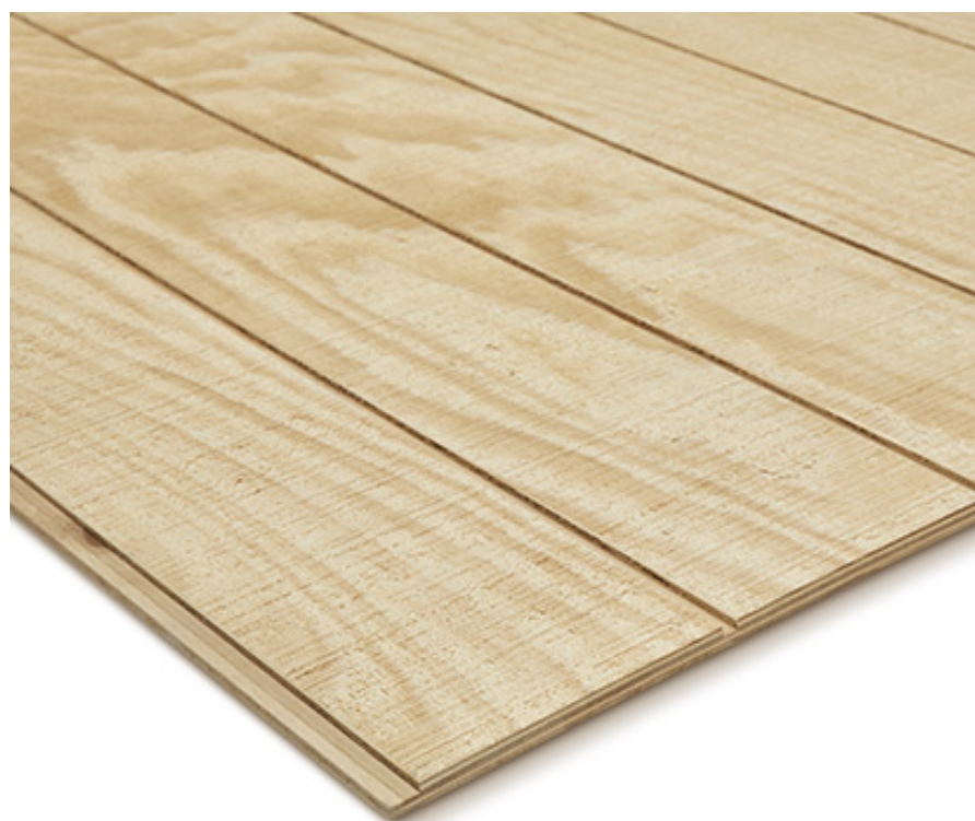
Dimensions (mm) 1220x2440 Thickness (mm) 12 15 Thickness (inches) 15/32 19/32 N° of layers 5 5 Density 480 - 550 kg / m 3 Sanding grain 150 grits on front and 120 grits on back Adhesive Phenol-formaldehyde that complies with E1 emission standard. Moisture content 8% to 12% Structural certification ANSI-APA PRP 210 & EN 13986 (CE2+) by HFB Forestry certification FSC® and PEFC™ certified products
